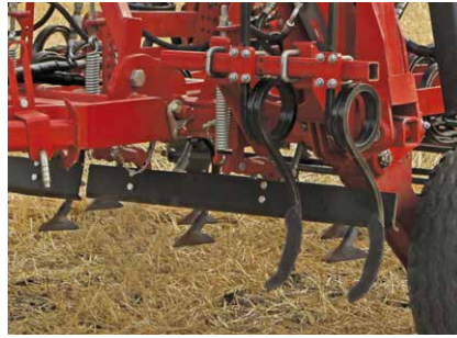
Loosened wheel tracks
